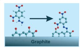
Identifying quinone-like species on the surface of graphitic carbon and multi-walled carbon nanotubes using reactions with 2,4-dinitrophenylhydrazine to provide a voltammetric fingerprint
